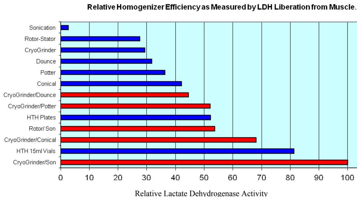
**Figure 20.** This relative efficiency chart is very revealing as regards the effectiveness of any single method on sample homogenization. The blue bars represent a single processing step while red bars are two-step processes.
