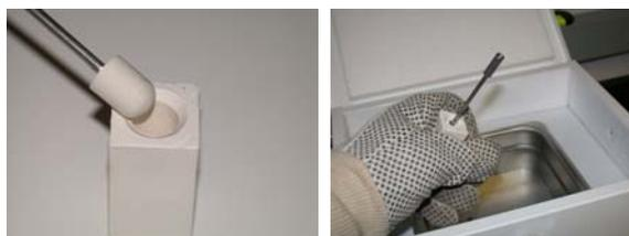
**Figure 2.** [CryoGrinder™](#) is useful for the cryogenic grinding of very small samples, less than 100 mg.
