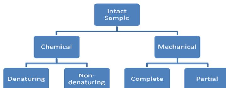
**Figure 1.** Simple schematic of sample disruption options. This simplified scheme does not consider that methods are normally combined during sample disruption. Mechanical homogenization normally makes use of buffers or lysis solutions just as chemical lysis normally requires that the sample contains small particles, which is normally created using a homogenizer.
