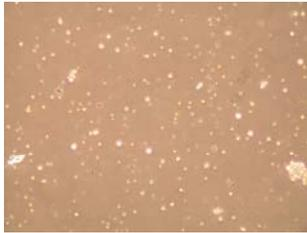
**Figure 11.** Though the homogenate appears very fine, significant tissue was left intact. The Dounce homogenizer produces 32% relative homogenization of solid muscle as compared to other processes (see Fig. 20).
