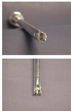
**Figure 8.** Top (upper) and side (bottom) views of a rotor/stator. The outer shaft (stator) remains stationary while the inner shaft (rotor) turns at speeds up to 20,000 rpm. Rotor/stators can be very effective on homogenizing powders and pills, but can generate only coarse homogenates when used on tougher tissues.
