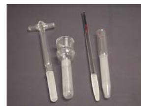
**Figure 6.** Tenbroeck (left) and conical (right) glass homogenizers.
