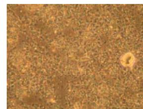
**Figure 16.** Cryogenic grinding followed by sonication proved to be the most efficient combination for homogenization with a relative efficiency of 100%. The density of small size of particles exceeded all other methods (see Fig. 20).
