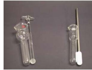
**Figure 10.** Two glass homogenizers used for shearing cells. The Dounce homogenizer (left) is manually operated and disrupts cells by forcing them between the pestle and tube wall. The Potter-Elvehjem homogenizer can be hand operated or attached to a motor. The pestle can be PTFE or glass.
