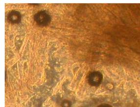
**Figure 7.** Mouse heart muscle homogenized with a blender. Blenders are an effective first step in disaggregating samples. However as depicted in this image, many microfibrils remain intact. Blenders can also introduce air bubbles (dark spots) which can be detrimental to some analytes.
