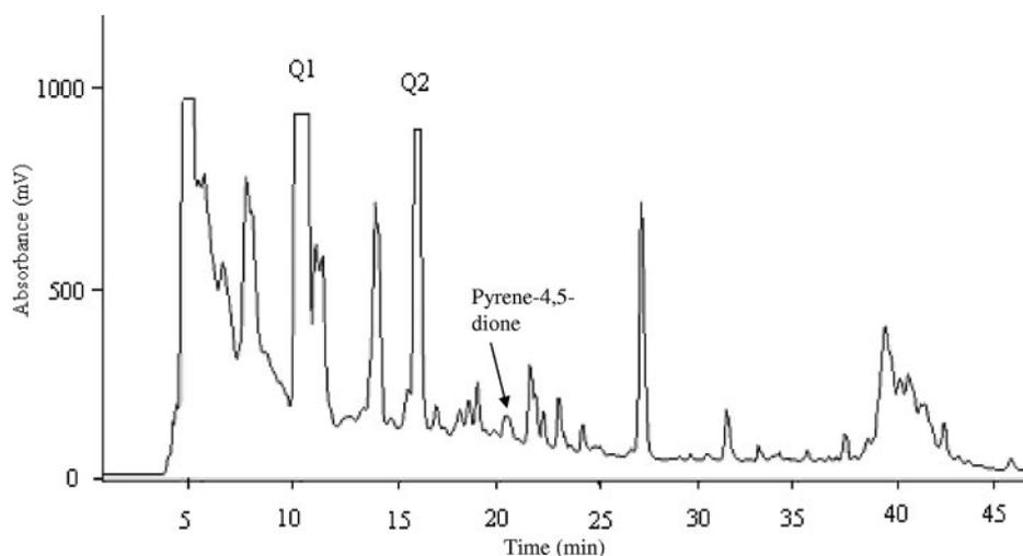
FIG. 2. HPLC chromatogram showing UV absorbance at 254 nm of an acidic extract from *Mycobacterium* sp. strain KMS culture with pyrene-4,5-dione added. The Q1 and Q2 fractions were obtained by using a semi-preparative HPLC column and were identified as phenanthrene-4,5-dicarboxylic acid and 4-phenanthroic acid, respectively.
