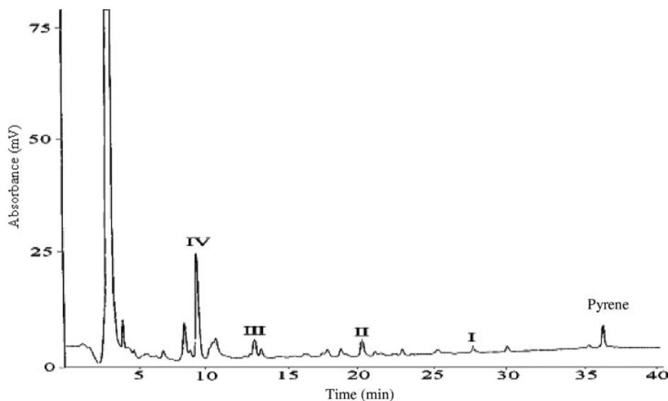
FIG. 1. HPLC chromatogram showing UV absorbance at 254 nm of CLLE-extractable pyrene residues in *Mycobacterium* sp. strain KMS culture after a 1-week exposure to pyrene. (I) 1-hydroxypyrene; (II) pyrene-4,5-dione; (III) *cis*-4,5-pyrene-dihydrodiol; (IV) phenanthrene-4,5-dicarboxylic acid.
